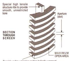
Special wedge wrapping section helically wrapped to form continuous non-clogging aperture
